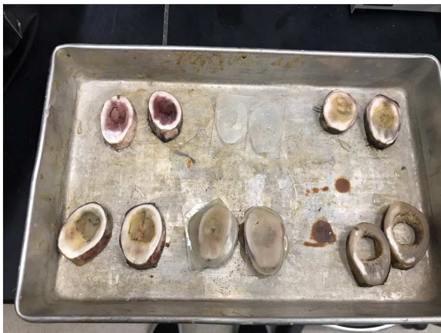
(Figure 2: From upper left to lower right: Frozen sample, Pre-control sample 1, Freeze-thaw sample, Control sample, Pre-control sample 2, Heat-simulated sample)
