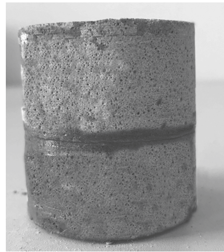
FIGURE 3: Test model to determine shear parameters of the surface of a grout-infilled flaw.
