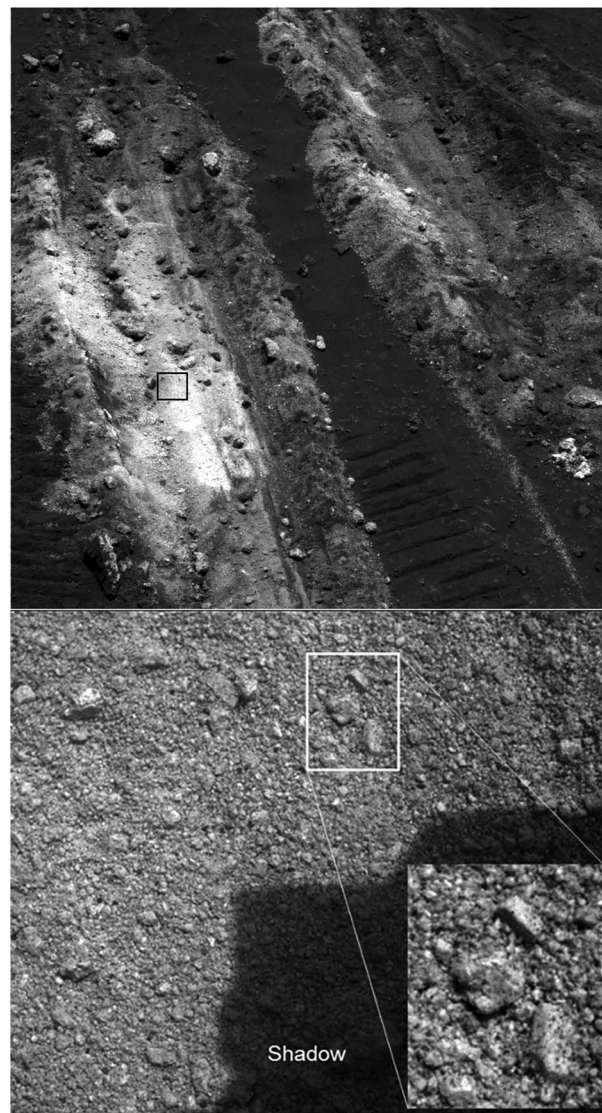
Figure 37. (top) Sol 1198 Pancam blue image 2P232715127EFFATB4P2539L7M1 of Gertrude Weise wheel track, with area shown below outlined in black. For context, see Figure 23a. (bottom) Part of Microscopic Imager image 2M231921836 of target Kenosha Comets, acquired on Sol 1189 with illumination from top. Full frame is \sim 3 cm across; inset shows 4.7 \times 5.8 -mm area. Note in inset that largest (very coarse sand) grains appear to contain dark grains in brighter matrix and wide range of clast sizes and shapes.
