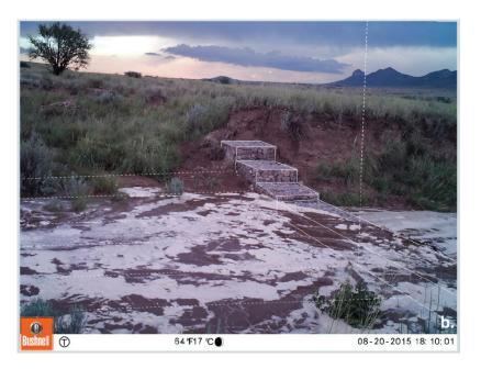
**Figure 6.** Photo taken 5 min after flow onset. Guidelines were superimposed later to assist in estimating ponding extent by C. Fandel.
