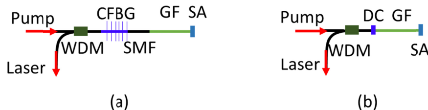
Fig. 1. The configurations of (a) a GHz repetition rate mode-locked AFL in which a CFBG is used as the output coupler and (b) a GHz repetition rate mode-locked AFL in which a fiber-optic dichroic mirror is used as the output coupler.
