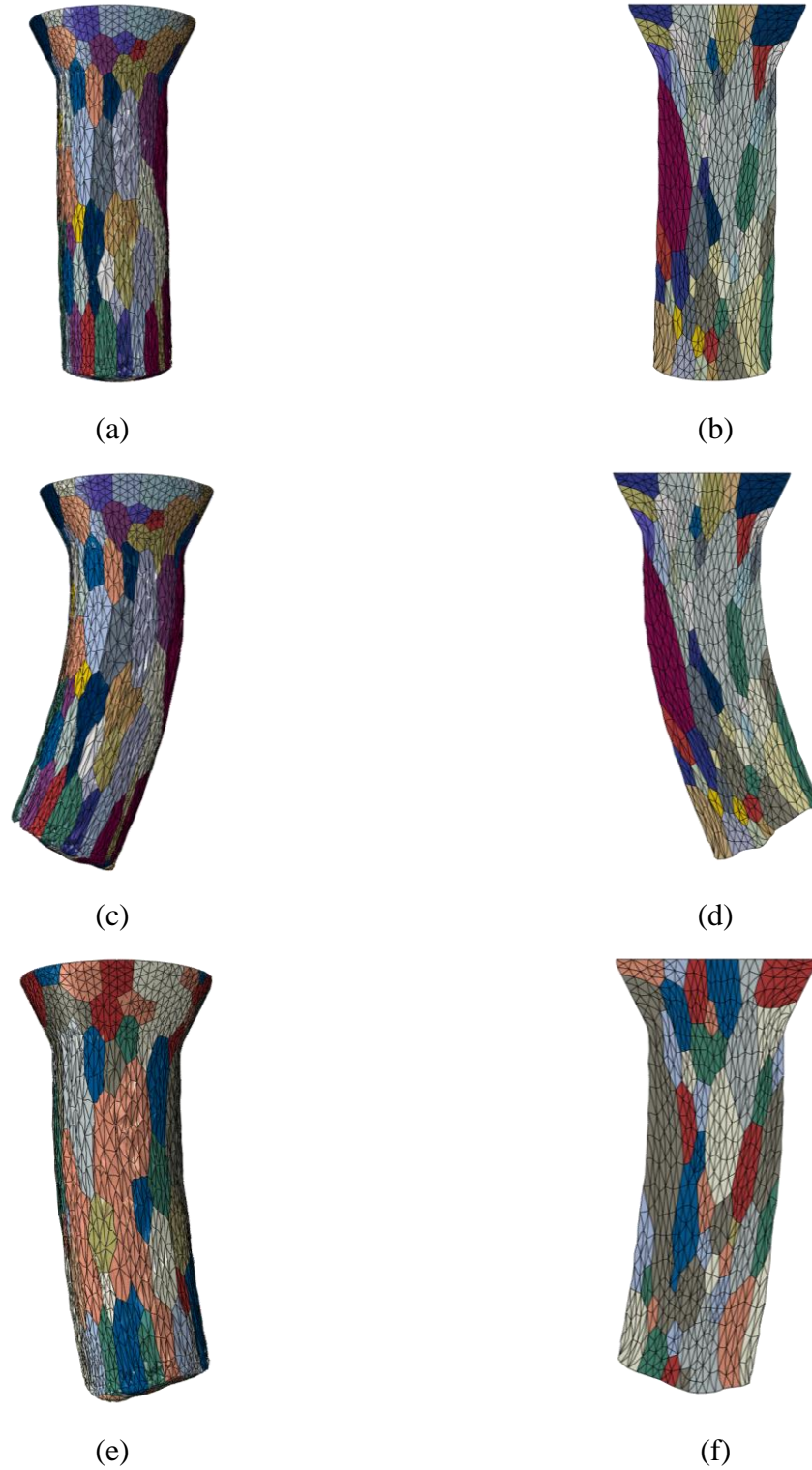
Figure 4.8: Grain morphology after extrusion: (a) front view (homogeneous), (b) rear view (homogeneous), (c) front view (set-1), (d) rear view (set-1), (e) front view (set-2), (f) rear view (set-2)
