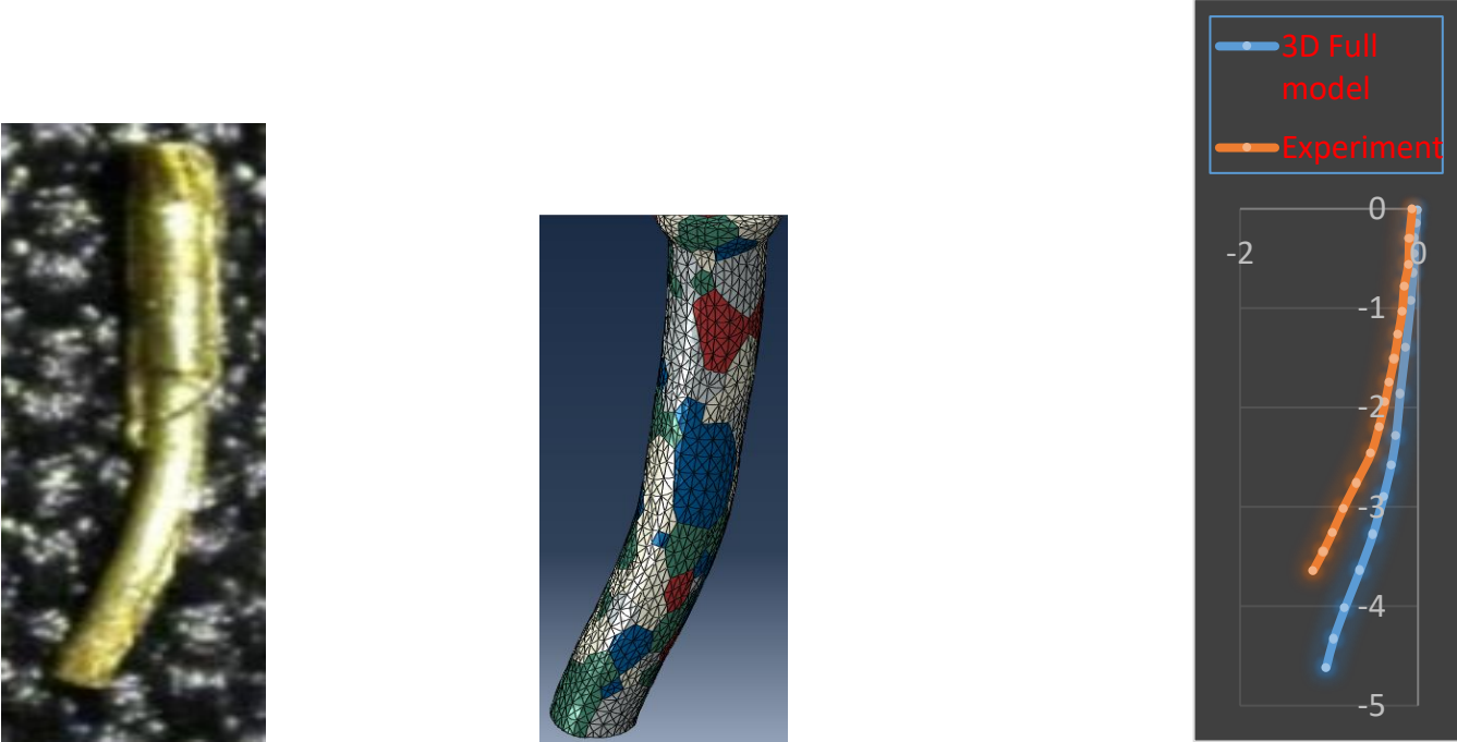
Figure 4.17: Comparison between experimental and computational deflection magnitudes (all units are in mm)
