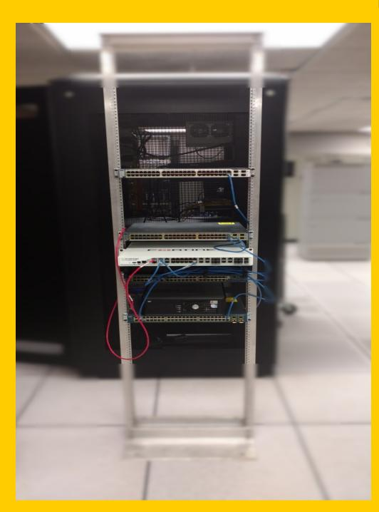
The test rack was assembled in the Kretzmann IT Data Center, utilizing retired components of our network infrastructure. This gives the test environment a comparable structure to that of the actual network infrastructure. The test environment is then kept isolated from any current equipment by keeping it offline. A simulated network is created utilizing multiple routers, switches, and a web server machine.
