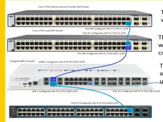
The top Cisco 3560 on the rack is the core switch of your local network which will be protected by your firewall and provide routing and access for all of the VLANs and devices on your local The top Cisco 3750 on the rack simulates a BGP router which would normally be located on the ISPs premises.
