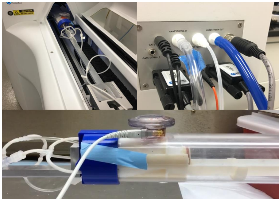
Figure 4. This figure shows the assembly of the device with vacuum and anesthesia lines connected in the rear and the AeroGen Pro mounted on top. This figure provides a detailed diagram of the device integrated into the Albira.
