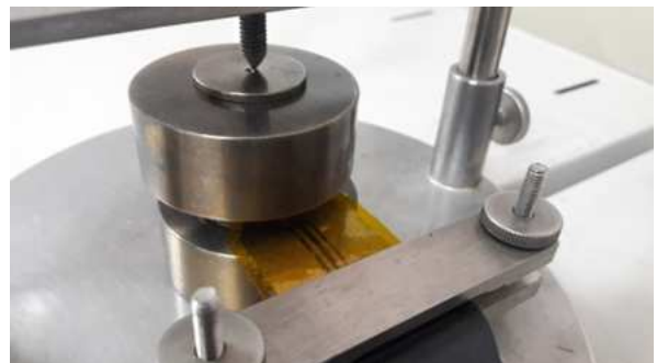
Fig. 2 Kapton® insulated sensor in between \phi 30 mm disc samples
