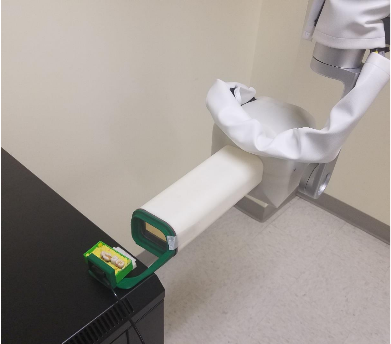
Figure 4. The s-IOT unit at the UNC School of Dentistry. Four teeth are mounted in a plastic Lego block using Play-Doh.
