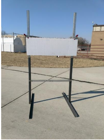
Figure 3.6 Obstacle used in the SCANSE Sweep test
