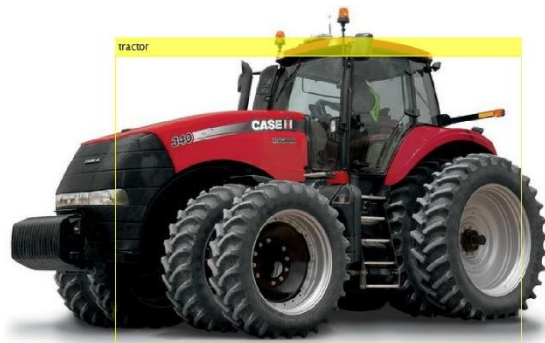
Figure 4.5 Viola-Jones algorithm detecting a tractor with no clutter. Yellow bounding box does not surround the entire tractor.
