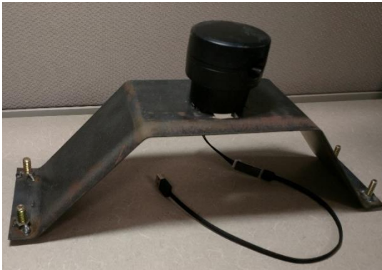
Figure 3.2 The SCANSE test stand with the spinning LIDAR mounted on the top the RPLIDAR. There was no trouble with data collection with the SCANSE, using the
