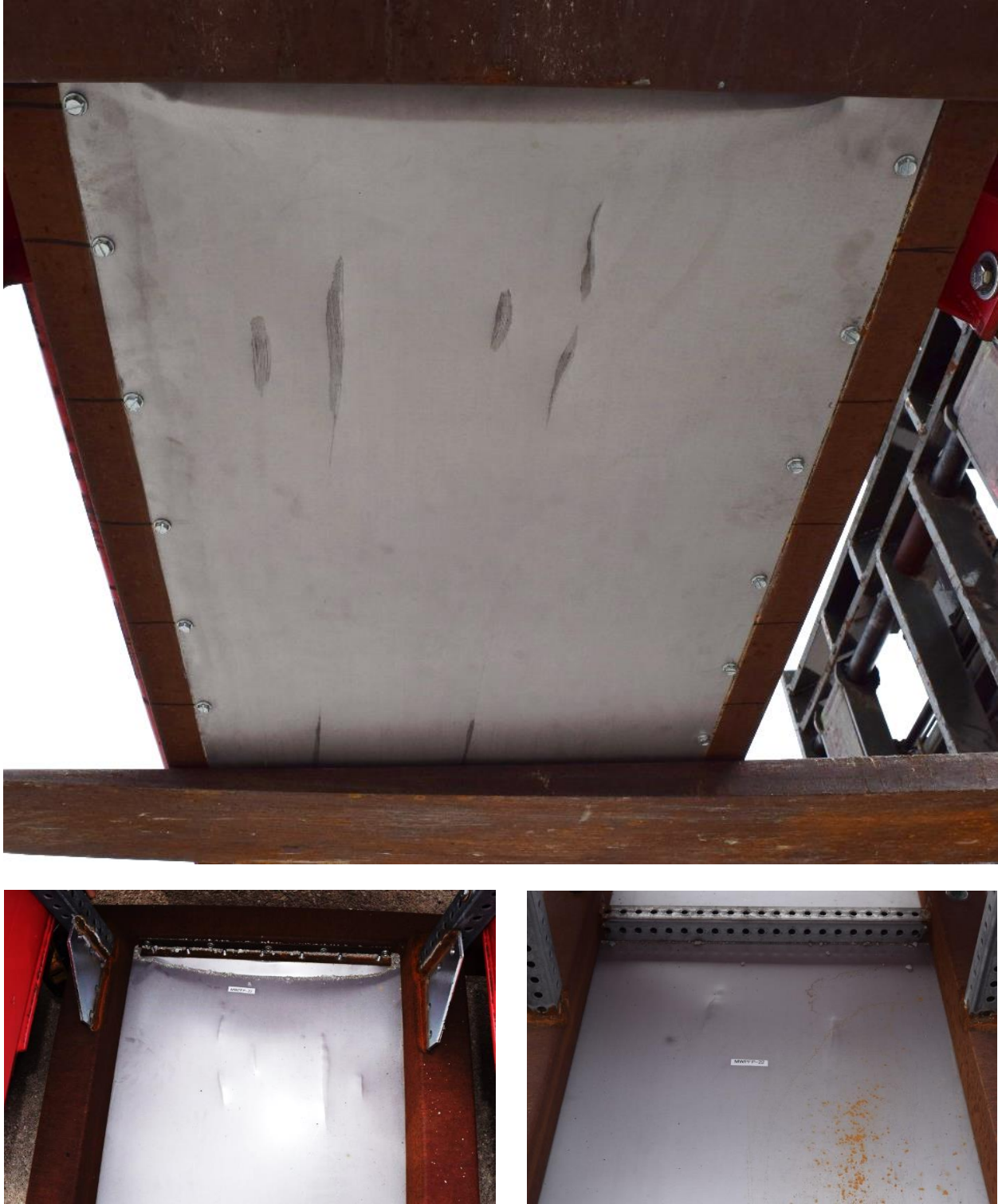
Figure 26. Simulated Floor Pan Damage, Test No. MWPFP-22
