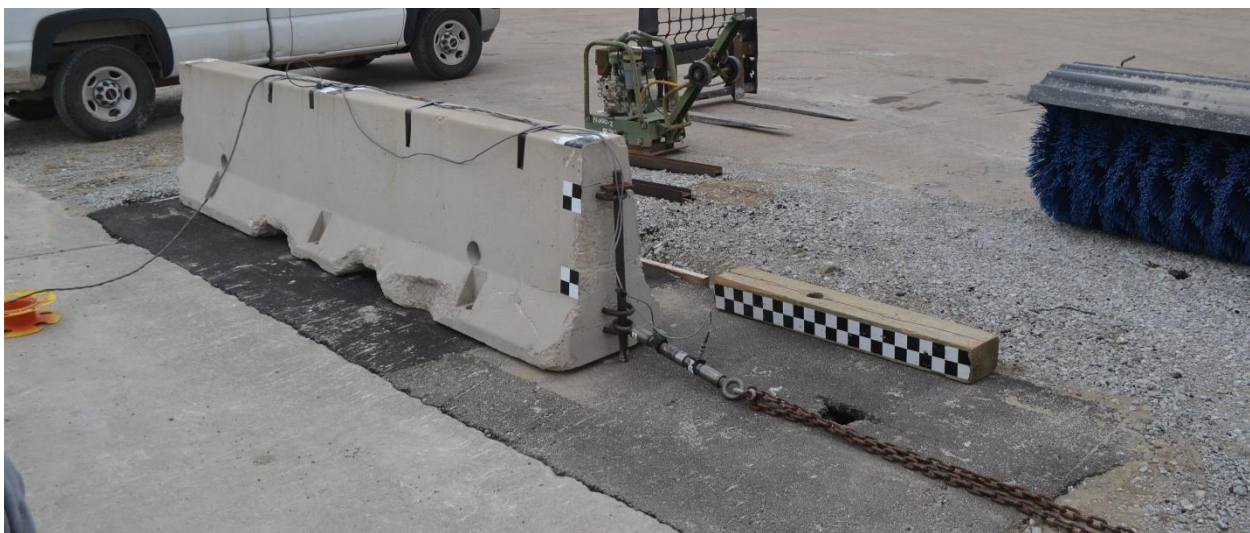
Figure 1. Quasi-Static Pull Test Setup, Test No. TCBFA-1
