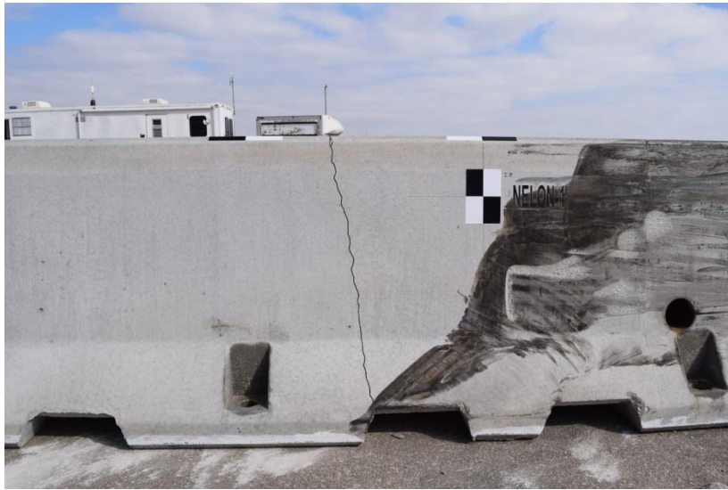
Figure 75. Barrier No. 3 Damage, Test No. NELON-1
