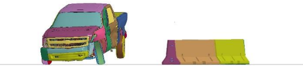
(d) impact US of joint between barrier nos. 12 and 13
