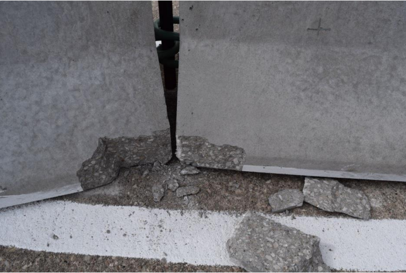
Figure 74. Barrier Nos. 1 and 2 Damage, Test No. NELON-1
