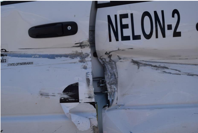
Figure 98. Vehicle Damage, Test No. NELON-2
