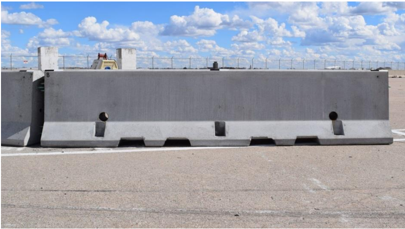
Figure 96. Barrier Nos. 7 and 8 Damage, Test No. NELON-2
