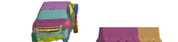
(e) impact US of joint between barrier nos. 13 and 14
