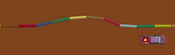
(h) impact US of joint between barrier nos. 8 and 9
