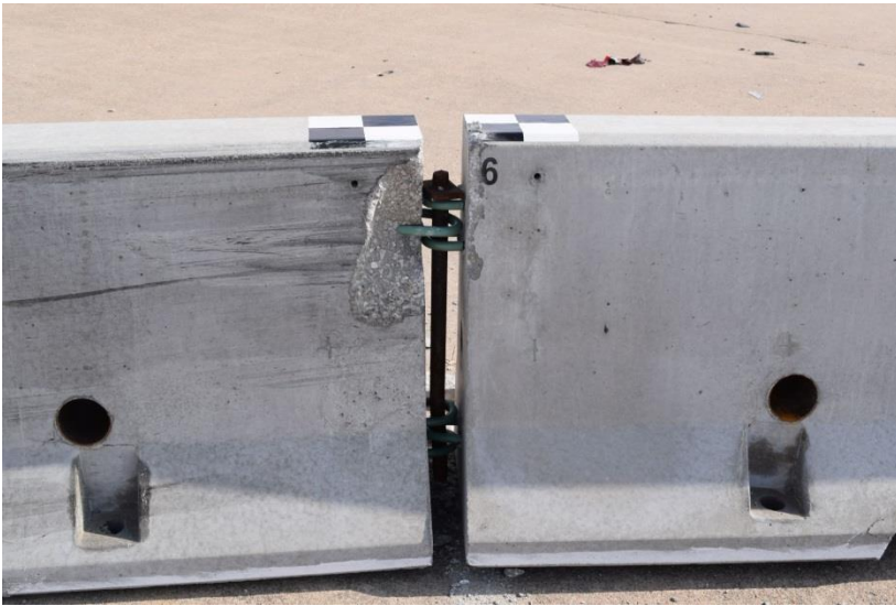
Figure 77. Barrier No. 5 Damage, Test No. NELON-1
