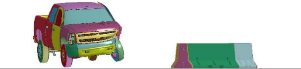
(b) impact US of joint between barrier nos. 10 and 11
