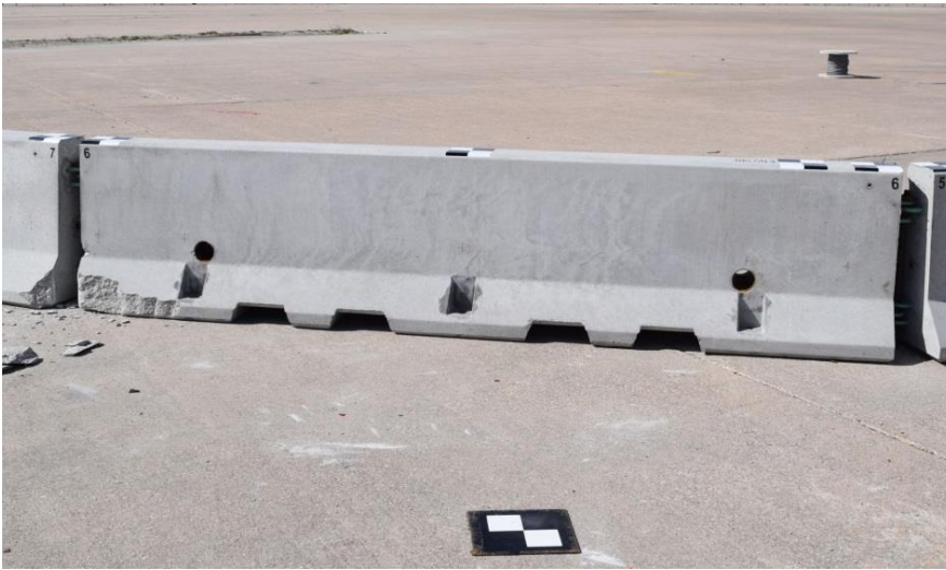
Figure 95. Barrier No. 6 Damage, Test No. NELON-2
