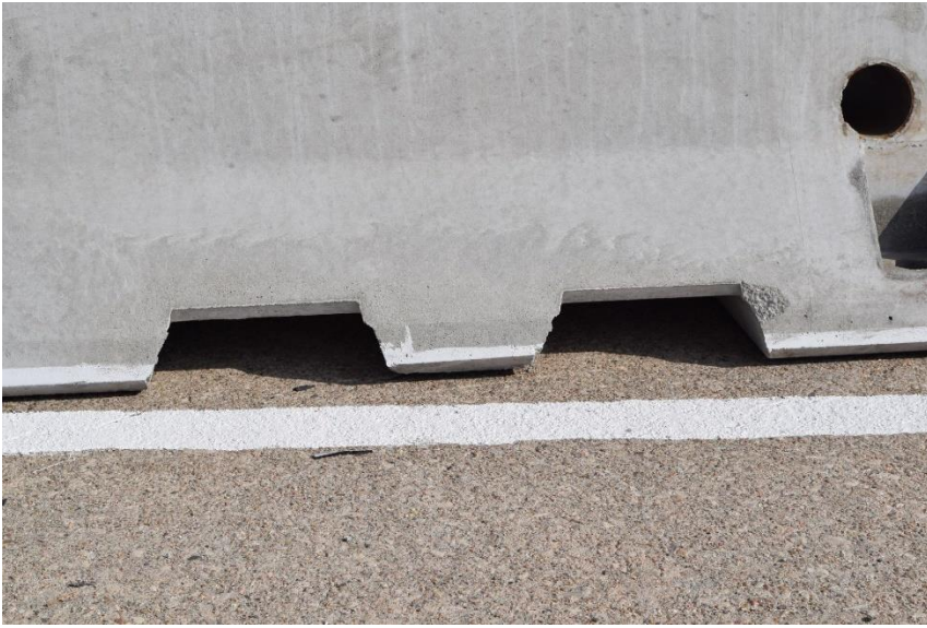
Figure 79. Barrier Nos. 7 and 8 Damage, Test No. NELON-1
