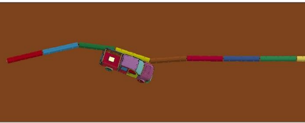
(b) impact US of joint between barrier nos. 2 and 3
