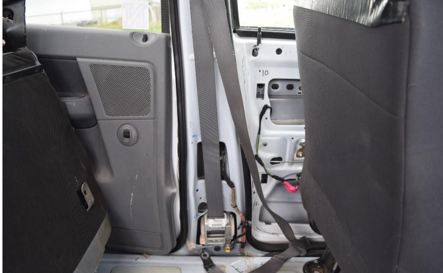
Figure 83. B-Pillar Deformation, Test No. NELON-2
