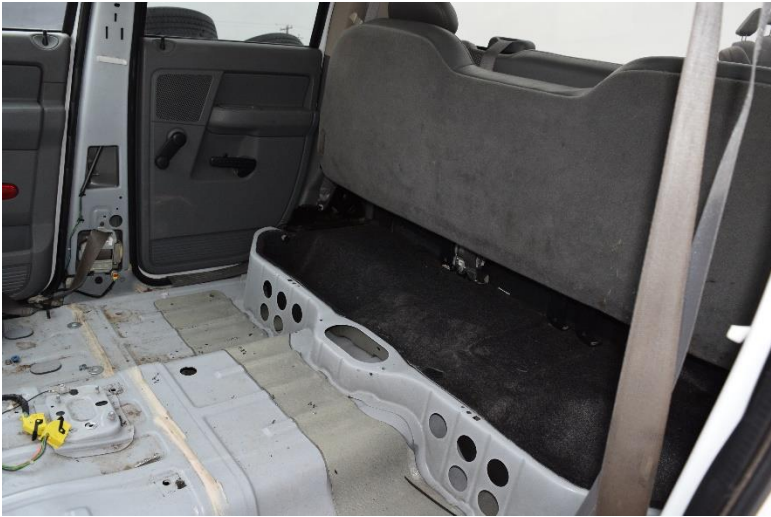
Figure 82. Occupant Compartment Damage, Test No. NELON-1
