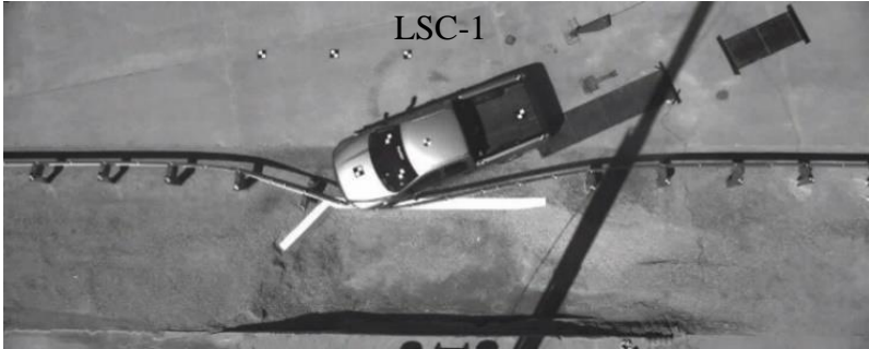
Figure 37. Overhead View at Time = 0.140 sec, Test Nos. MGSL-2, MGSMP-1, and LSC-1
