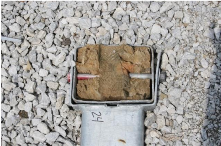
Figure 8. Post-Test Photographs of End Anchorage System, Test No. MGSLs-2
