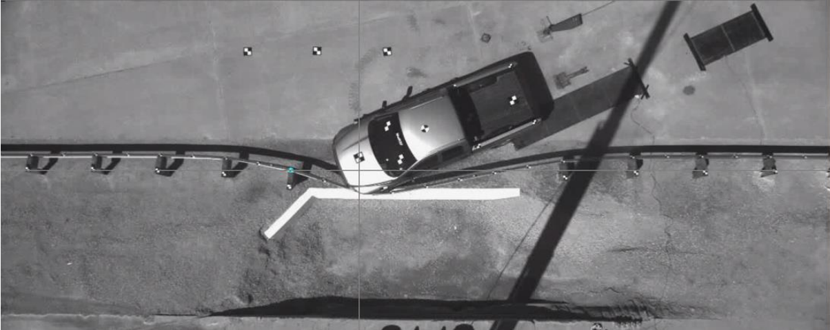
Fracture of First CRT Downstream of Unsupported Span
