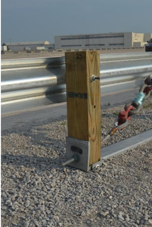
Figure 3. Long-Span End-Anchorage System, Test No. MGSL-2
