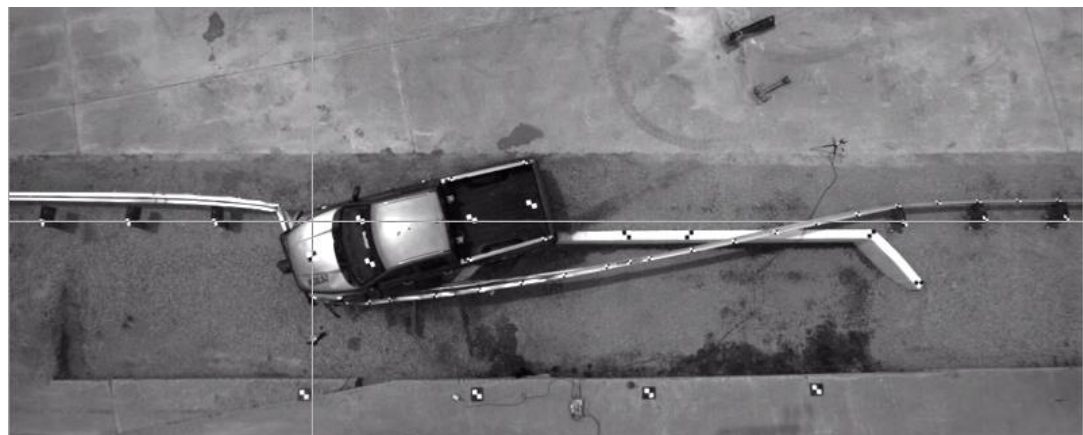
Fracture of Third UBSP Downstream of Unsupported Span
