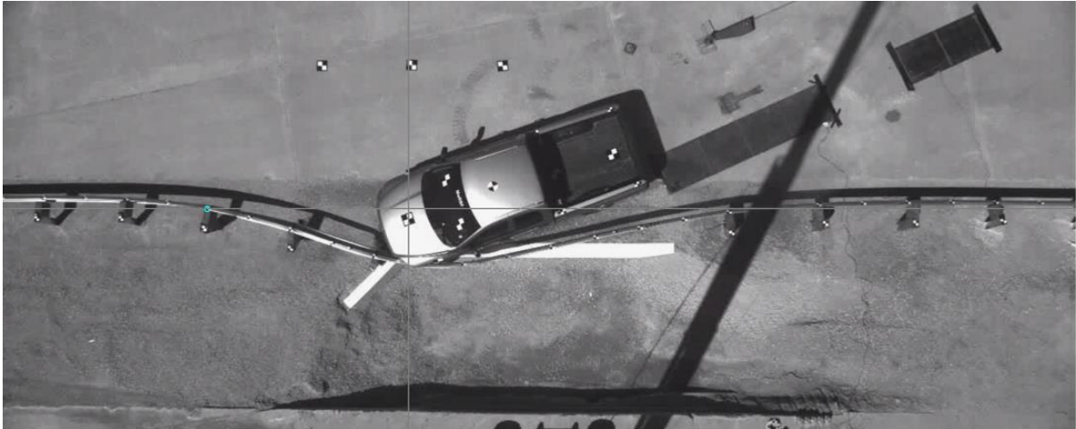
Fracture of Third CRT Downstream of Unsupported Span
