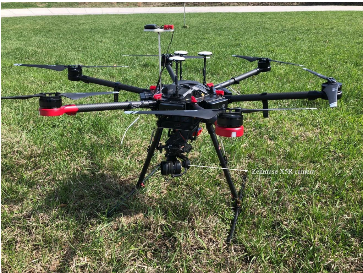
Figure 2.2. The DJI Matrice 600 pro UAV platform with Zenmuse X5R sensor used in this study.
