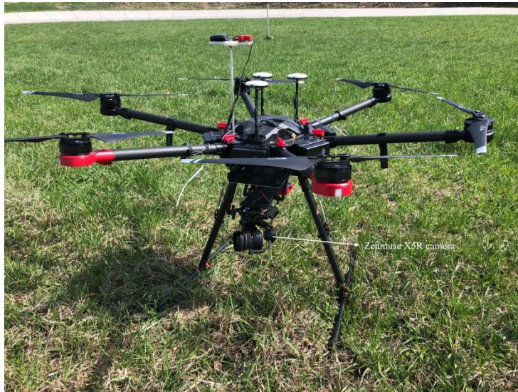
Figure 3.2 DJI Matrice 600 pro UAV platform with Zenmuse X5R camera
