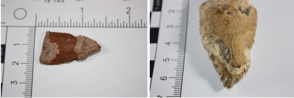
Figure 7.25 Pictures of the SHSC weathering along with some extreme breaking up of the material (Photo by author, collection of the U.S. Department of Interior, Bureau of Reclamation)
