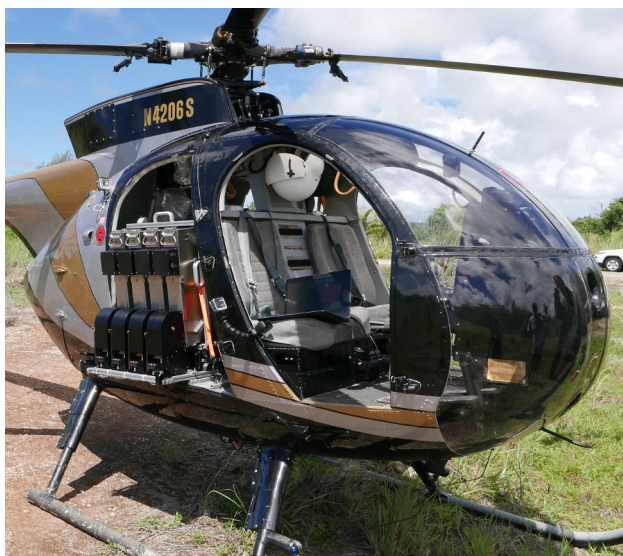
Fig. 5 Complete ADM with loaded magazines mounted in a McDonnell-Douglas MD 500D helicopter.
