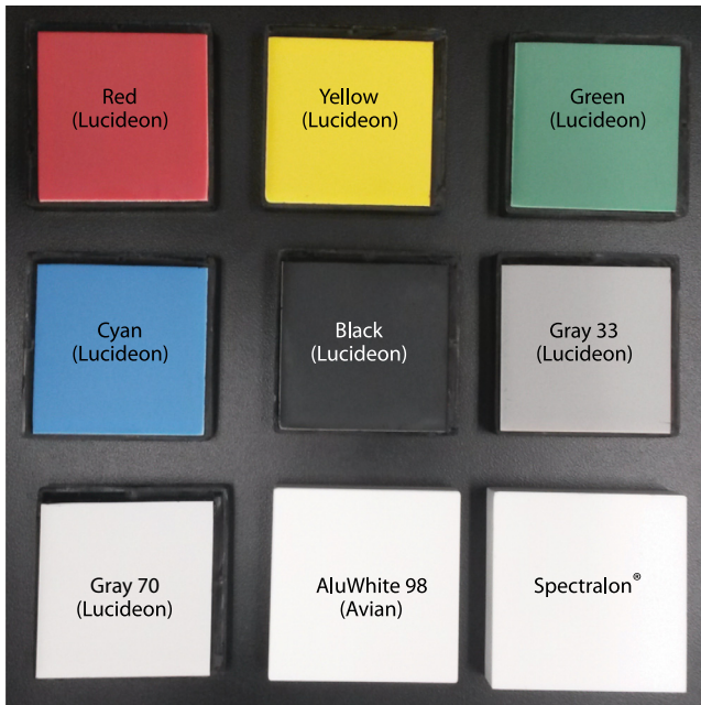
Fig. 4 Calibration targets used in this study with manufacturer indicated in parentheses and Spectralon® for comparison. All of the Lucideon targets are mounted on a black plastic holder. The white target is not mounted.
