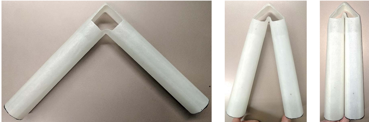
Figure 11. Fourth iteration FRP joint in fully deployed, partially folded, and fully folded configurations.
