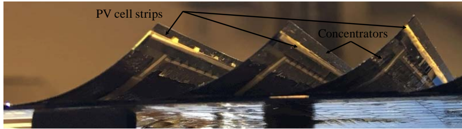
Figure 5. Solar cell strips attached to the back of concentrators.
