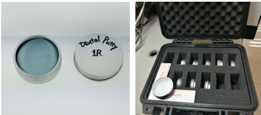
Figure 6. A container system for the storage and transportation of delicate plastic prints. A piece of dental silicone putty (left) containing a thumb impression was stored in a 5 mL aluminum container, which was placed in a Pelican™ 1200 case (right) for storage and transport. Cardboard backing was used for materials of limited quantity.
