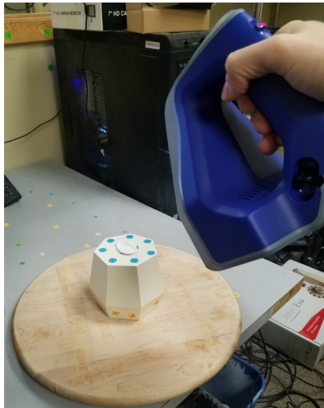
Figure 12. Scanning of a 3D fingerprint impression using a handheld structured-light 3D scanner. The impression was taken out of its container and placed on a stand with reference markers. A turntable was used to adjust scan angles while the scanner was held still. The photograph was supplied courtesy of Laser Design, Inc.
