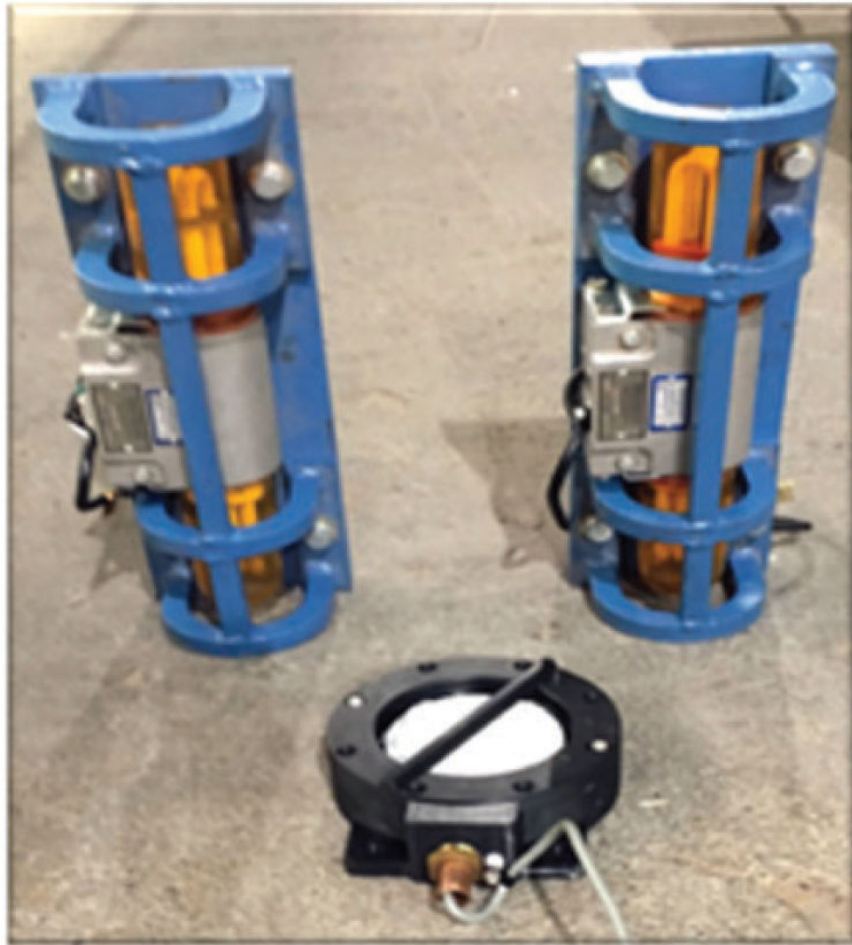
Figure 5. The Saturn luminaire pictured next to two existing roof bolter CFL luminaires
