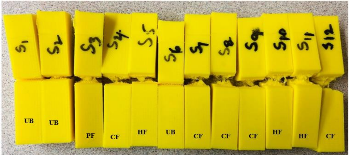
Figure 19.Types of failure of twelve impacted specimens
