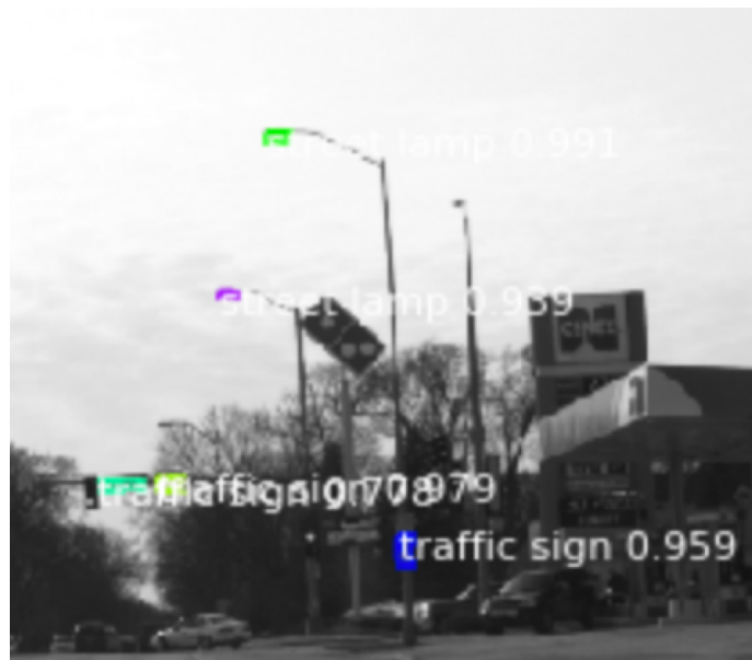
Figure 5: The part of result of the day image on Mask RCNN
