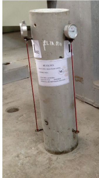
Fig 11. Arranging measuring indicator on specimens without load
