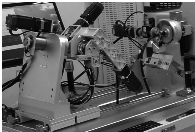
Fig. 1. The slave robot mounted on conventional colonoscope (arrow), and robotic arm (*) holding control body of colonoscope.
