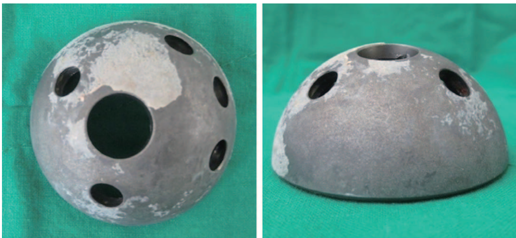
Fig. 4. The acetabular cup, which was retrieved at 4 years after index operation, showed extensive loss of hydroxyapatite coating.
