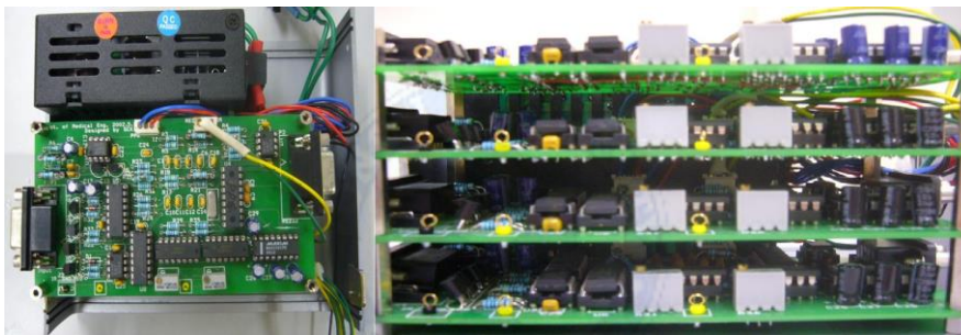
Fig. 11. A photo of 4-ch photoplethysmography measurement device.
