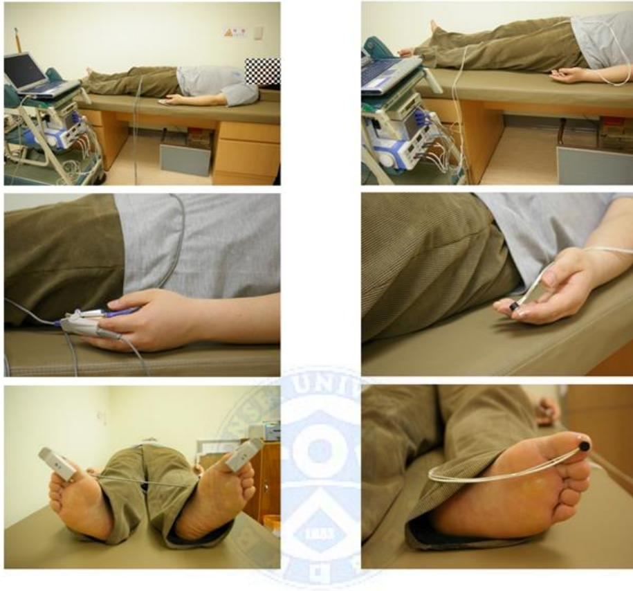
Fig. 17. A photo of measurement using the PPG and LD devices.
