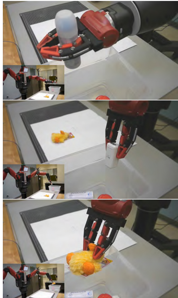
Fig. 18 Packing a box with random objects using power and precision grasps (still frames from the linked video)
