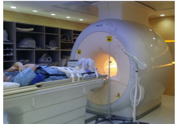
Fig. 1 Axial loading experiment apparatus mounted on the magnetic resonance imaging table
