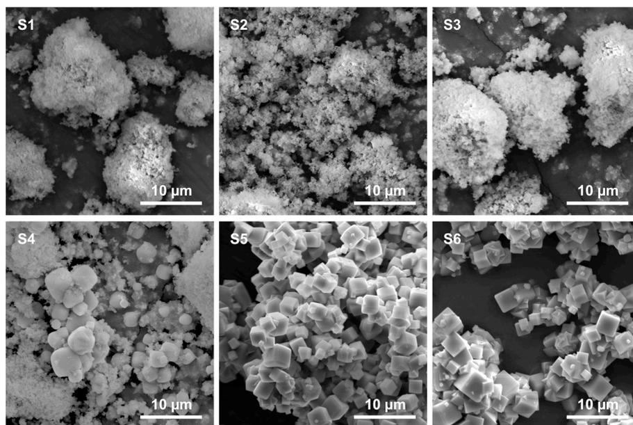
Fig. 3. SEM images of the six collected in-process samples according to Fig. 2 after 0.25 h (S1), 0.75 h (S2), 1.25 h (S3), 2 h (S4), 2.67 h (S5), and 3.08 h (S6).
