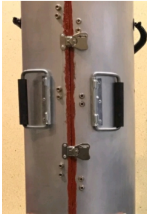
Figure 28: Silicone rubber sheets compressed with the latches to provide a tight seal.
