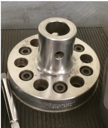
Figure 35: Instron machine mount point. Cylindrical grips are inserted and pinned into place.
