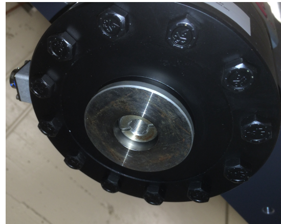
Figure 36: MTS machine mount point. Cylindrical threaded grips are screwed into place.
