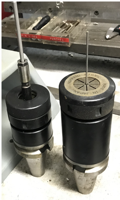
Figure 39: Large tool holders for 2 mm and 5 mm wires.
