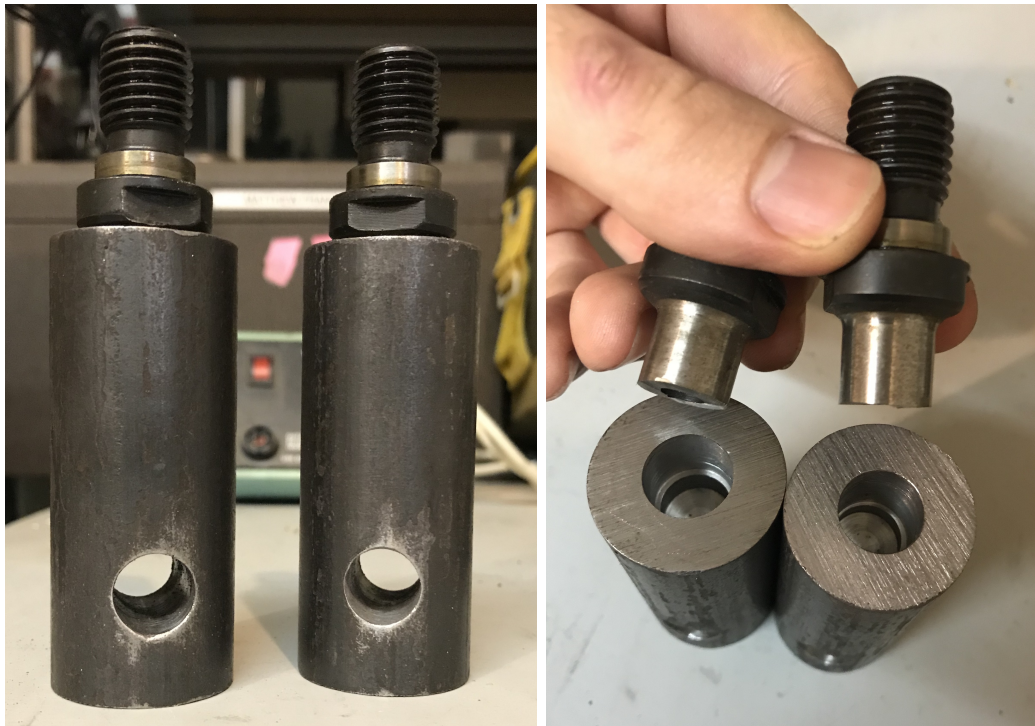
Figure 40: Machined adapters for large tool holders, prior to welding and finishing. Work was performed by our sponsor Digital Loggers, Inc.
