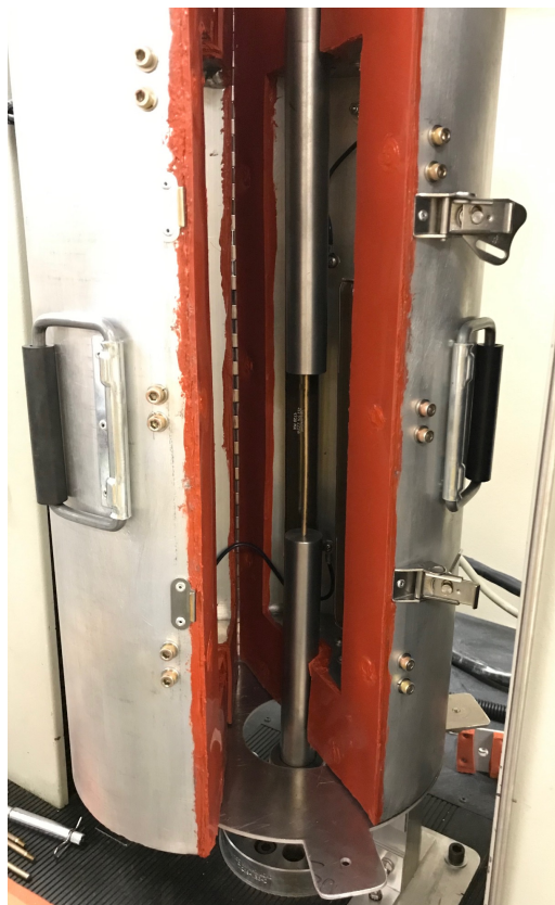
Figure 45: Grips and specimen installed with the environment chamber.
