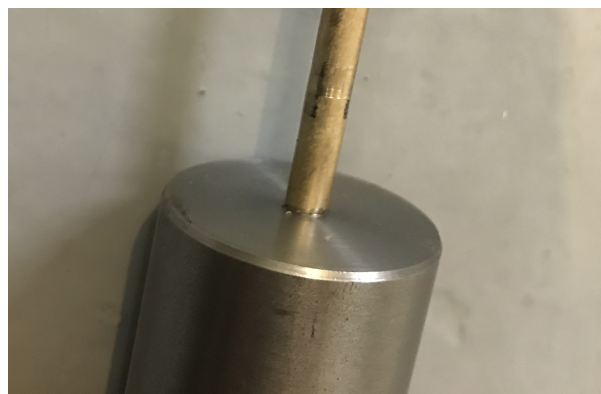
Figure 43: Grip fitment with specimen.
