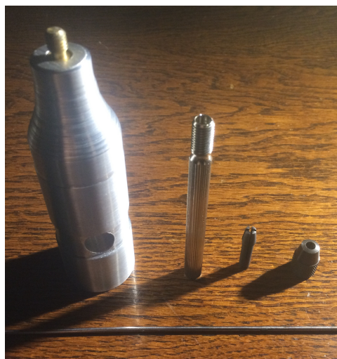
Figure 37: Prototype collet grip - disassembled.
