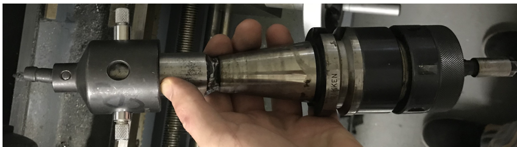
Figure 41: Completed specimen fixturing for the Instron machine. An adapter, tool holder, and collet are used to grip narrow wire specimens of 2 mm or 5 mm diameter.
