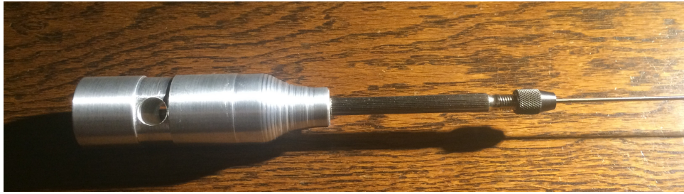
Figure 38: Prototype collet grip - assembled.
