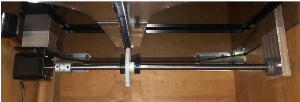
Figure 19. Transmission subassembly, side view of gear interface
