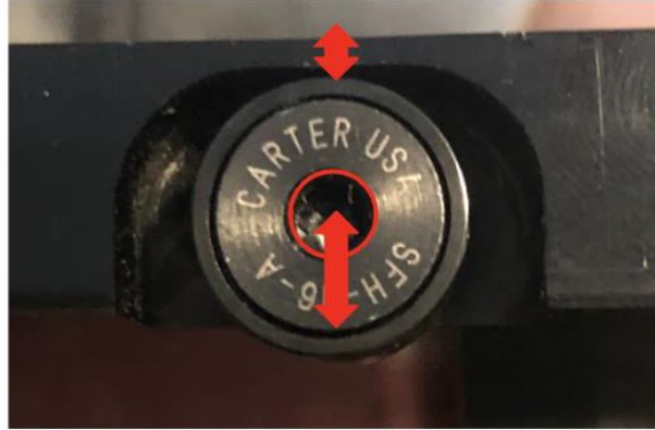
Figure 24. Track roller hub design showing thin features
