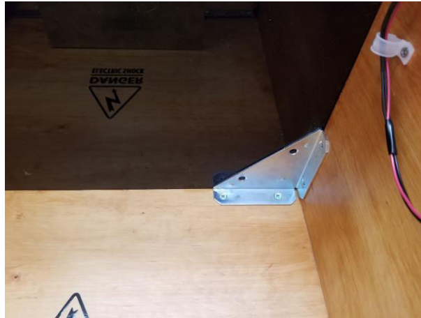
Figure 9. Angle Bracket Supporting Lid Subsystem
