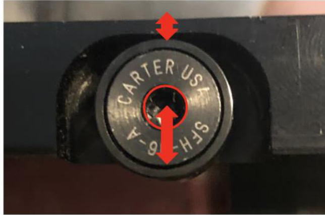
Figure F1. Track roller in door showing hub and thin features
