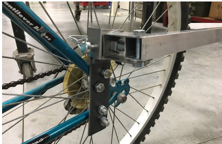
Figure 61. A manufactured implementation of the hitch locking mechanism.
