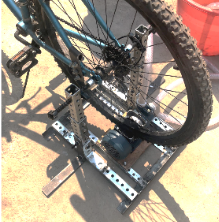
Figure 37. Kickstand Attached to Rear Axle of Bike with Pump and Removable Stabilizers
