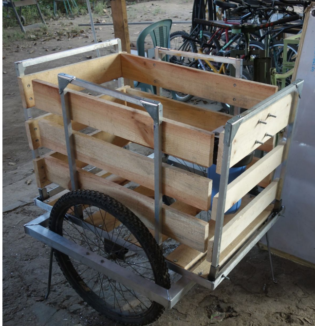
Figure 49. Final constructed cart with the kickstand visible.
