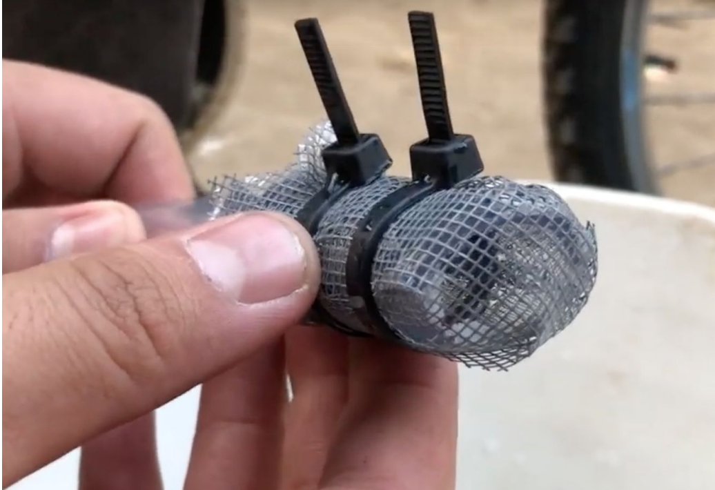
Figure 30. Fine Mesh Pre-Filter at Inlet of Tubing
