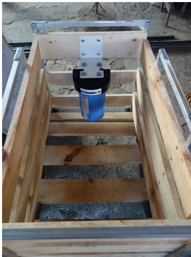
Figure 50. Final constructed cart with the purification module and holder visible.
