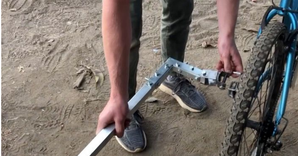
Figure 65. Extension of Hitch Connection between Bike for Increased Turning Radius
