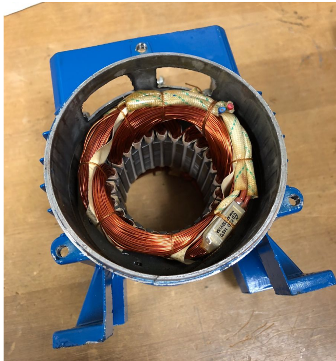
Figure 27. Inside of Pump Housing Prior to Removal of Inner Magnetic Components
