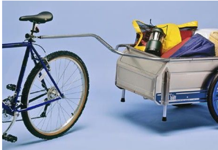
Figure 19. The seat rod connection mechanism for attaching the cart to a bicycle [20, Reproduced w/o permission]
