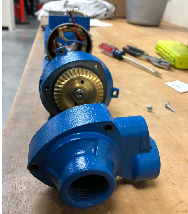
Figure 26. Exploded Front View of Pump with Exposed Impeller Blade
