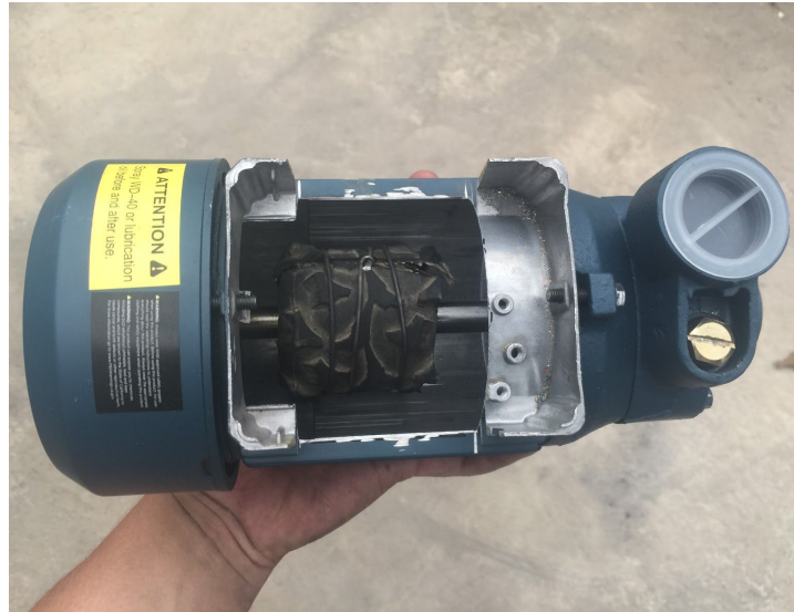
Figure 28. Mechanically Converted Centrifugal Pump in Guatemala
