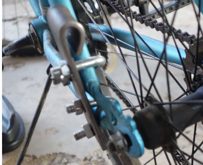
Figure 63. \frac{1}{8} " Bent Steel Plate Connected with \frac{5}{8} " Cable Clamps with PTO Pin Slot
