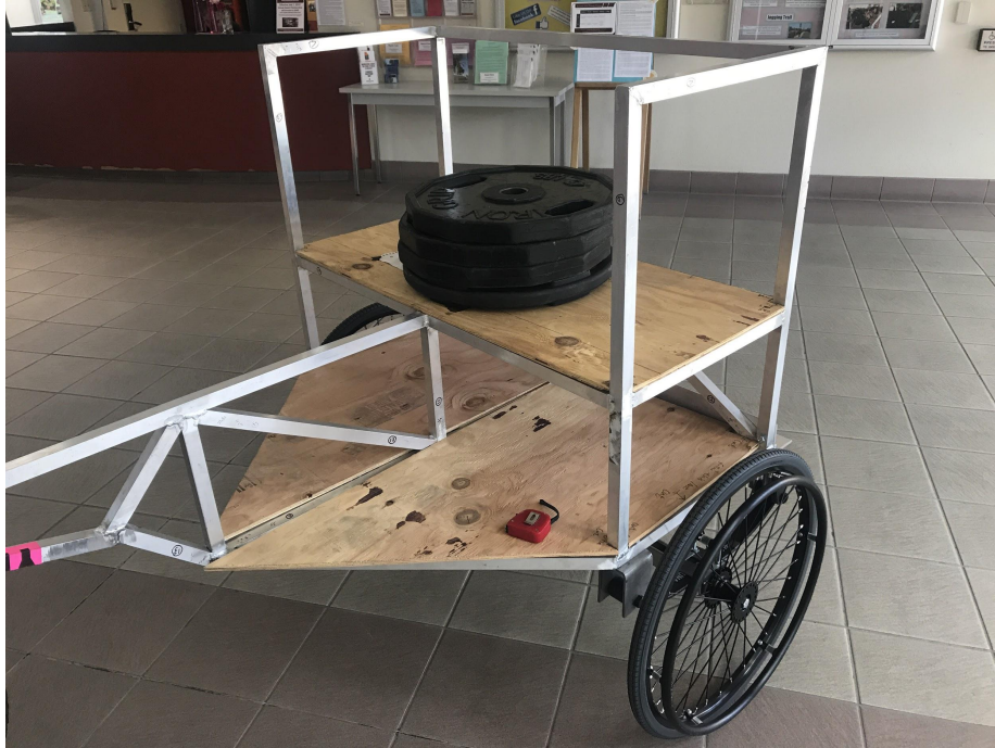
Figure 51. Static loading testing at Malley Recreation Center at SCU.
