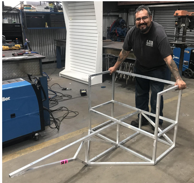
Figure 16. The BiciTaxi frame, welded by Juan from Yes Welding.
