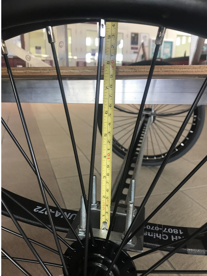
Figure 50. Deflection test for 225 pounds of load.
