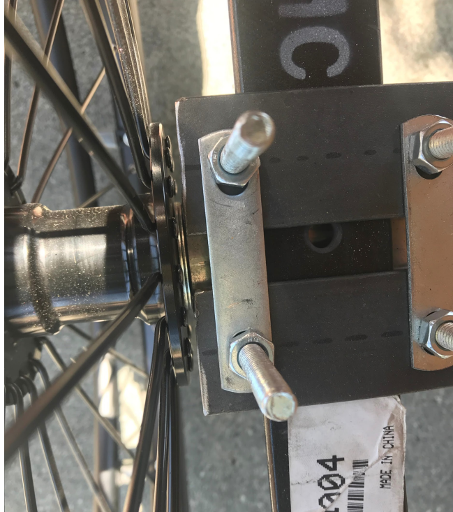
Figure 26. Clearance between U-bolt straps and wheels.
