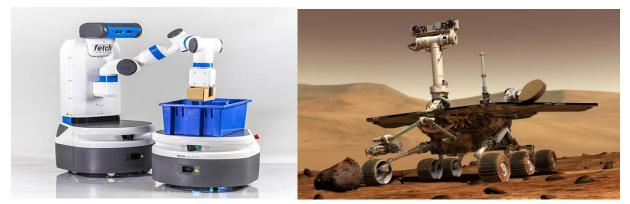
*Figure 3*. Fetch Mobile Manipulator [5] *Figure 4*. NASA Opportunity, a mobile sensor suite [6]
