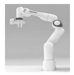
Figure 1: Franka Industrial Manipulator w/gripper [2]
