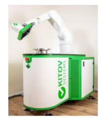
Figure 2: Kitov System - Denso Robot w/ Camera [3]
