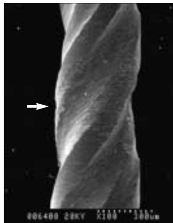
Figure 3. A SEM image of surface defect (arrow) of K3™ (experimental group, ×150).
