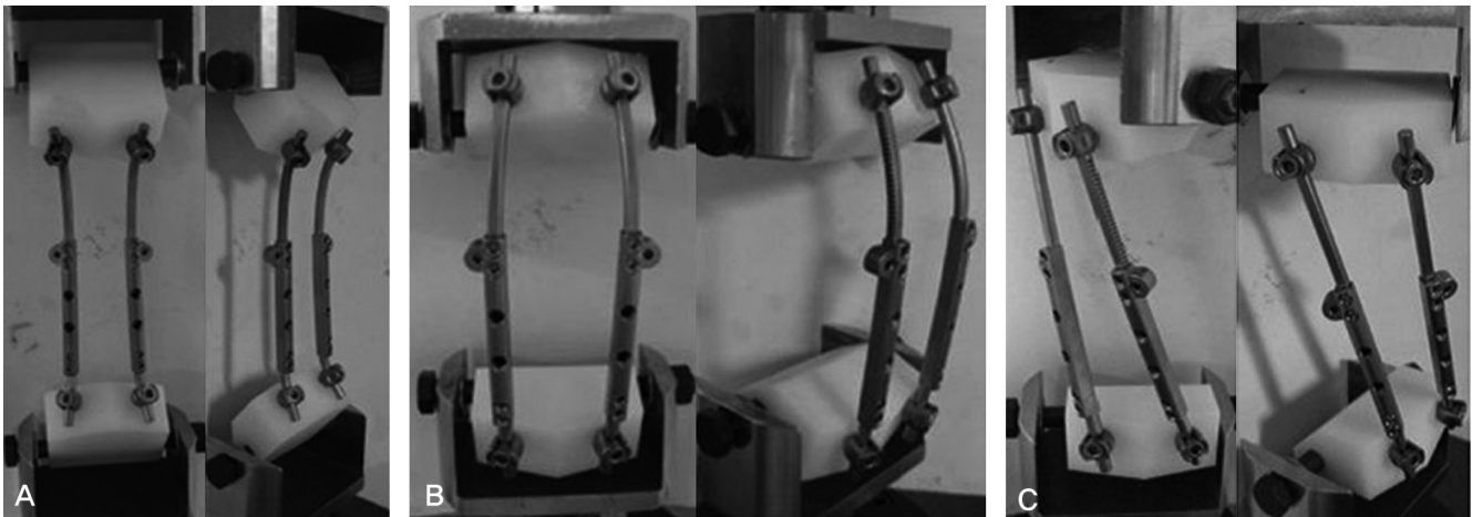
Fig. 4. These pictures show the test results of growing rods construct during the extension test (A), the compression test (B), and the torsion test(C).
