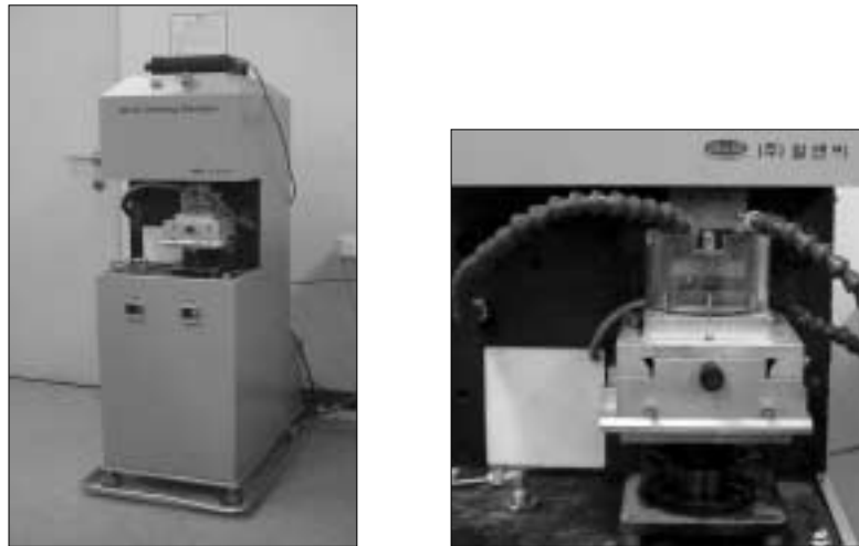
Figure 6. Chewing simulator (R&B, Daejeon, Korea).
