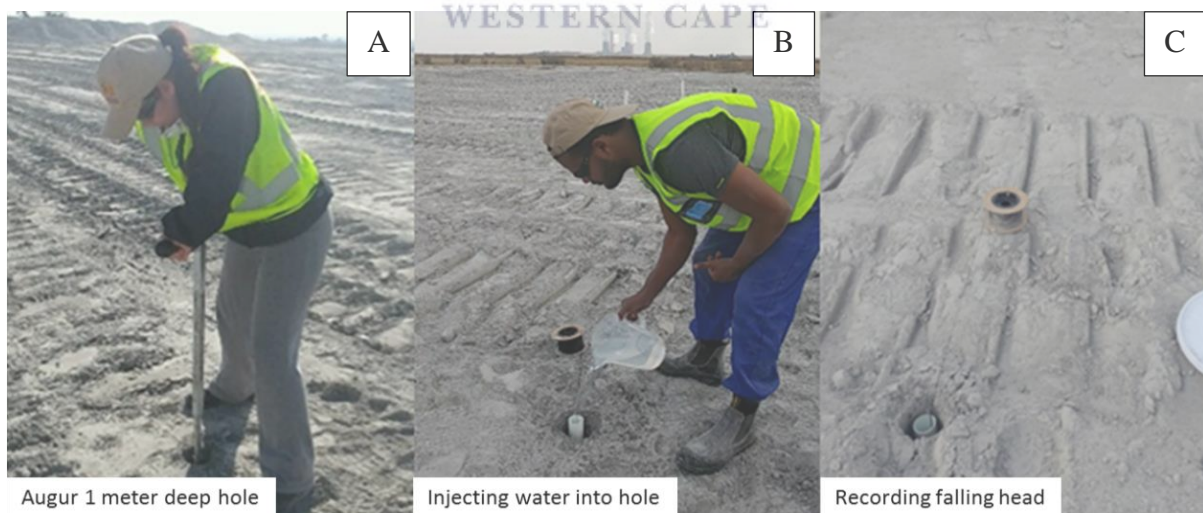
FIGURE 3.3. Falling head hydraulic test procedure on fly ash dumps where (A) auger holes are drilled, (B) water injected into the hole with piezometer installed and, (C) falling head is recorded with a water level recording instrument.
