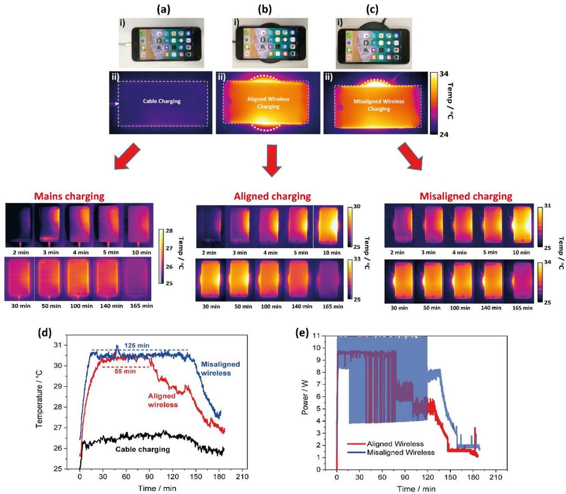
**Figure 4. Thermal imaging of the three modes of iPhone 8 Plus charging: (a) (i) Mains-driven cable charging, (b) (i) wireless charging where the phone coil is aligned with the coils of the charging base and (c) (i) where the coils are misaligned. (a-c) (ii) show the thermal profiles of the phone after 50 minutes of charging. (d) Graph show the temperature variation with time for the different modes of charging and (e) shows the power input during charging.**
