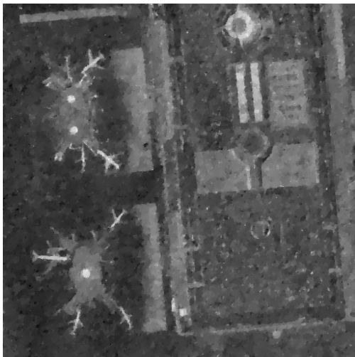
Figure 7. Recovery of coefficients by taking the median from correctly received channels. Reconstructed quality in PSNR = 22.044 dB.
