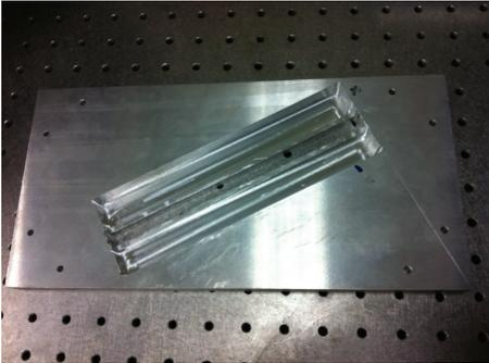
FIGURE 2: Picture of the diagonal groove rigid plate model.
