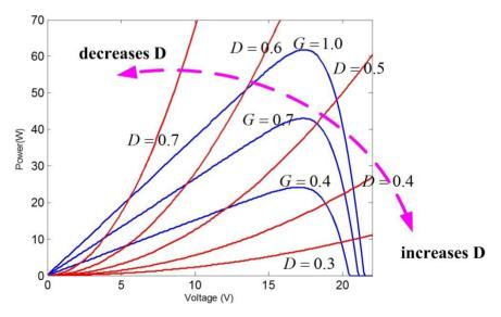
Figure 13. Power characteristics of the PV system.
