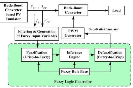
Figure 14. Fuzzy logic controller for the MPPT design.
