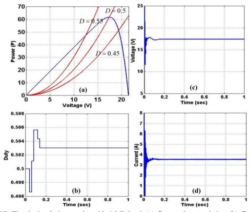
Figure 18. Circuit simulation results with  $4.9 \Omega$  load. (a). Power characteristics. (b). Duty ratio command. (c). Output voltage from PV emulator. (d). Output current from PV emulator.
