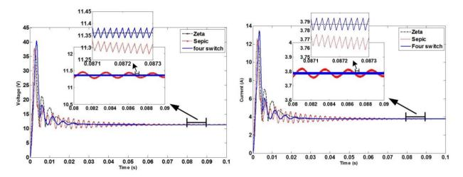
Figure 9. Voltage and current outputs from PV emulator for different buck-boost converter topologies loaded with  $3\Omega$  resistor.
