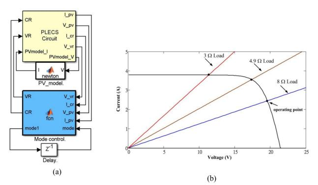
Figure 7. (a). Block diagram of the circuit simulation for the buck-boost converter based PV emulation system. (b). I-V characteristics of the PV panel and its corresponding operating points with different resistive loads.
