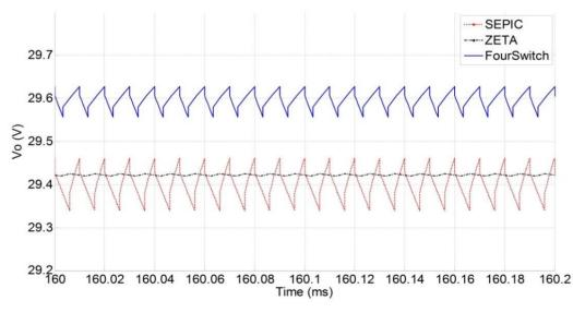
Figure 4. Comparison for steady-state responses
