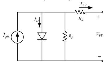
Figure 1. Single-diode equivalent circuit model
