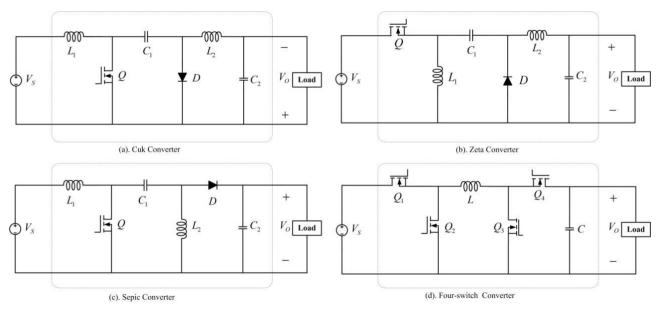
Figure 2. Buck-Boost Converters. (a). Cuk converter, (b). Zeta Converter, (c). SEPIC Converter, (d). Four-switch type converter.
