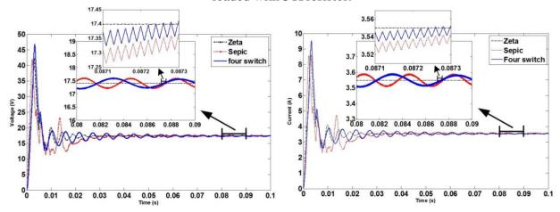
Figure 10. Voltage and current outputs from PV emulator for different buck-boost converter topologies loaded with  $4.9 \Omega$  resistor.
