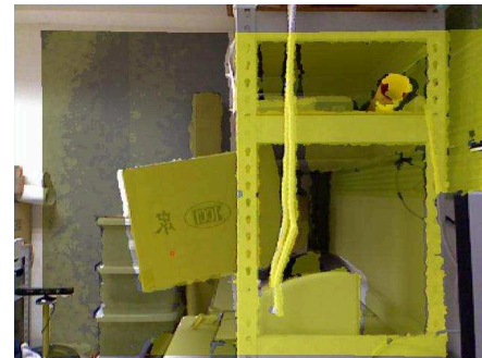
Fig. 5 Overlap image of Kinect RGB image and depth image
