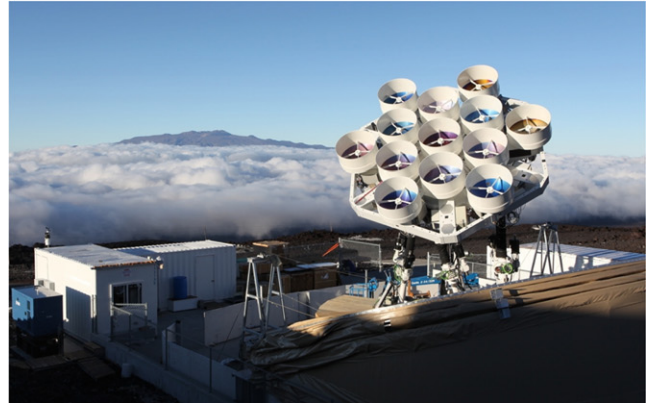
Figure 1. Pictures of AMiBA-7 (left) and AMiBA-13 (right). The antennas (0.6 m for AMiBA-7 and 1.2 m for AMiBA-13) and receivers are mounted in a compact configuration on the 6 m platform.
