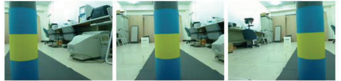
Fig. 17: With the same distance from the robot to the landmark, the (F_H, F_V) of the landmark at left, middle, and right positions of the frame are (86,227), (80,219), (87,223) pixels, respectively.
