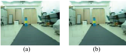
Fig. 15: The landmark images with distances of (a) 410cm and (b) 450cm. The (F_H, F_V) are equal to (a) (14,38), (b) (14,38) pixels in the frame.
