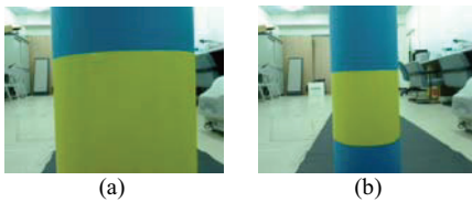
Fig. 14: The landmark images with distances of (a) 30cm and (b) 50cm. The (F_H, F_V) are equal to (a) (104,238), (b) (155,238) pixels in the frame.
