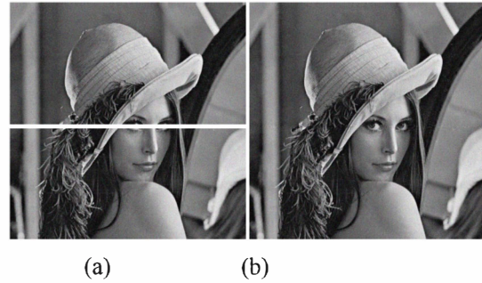
Fig. 5 (a) Damaged rate is 1.76% for Lena; (b) Restored image, PSNR=47.80
