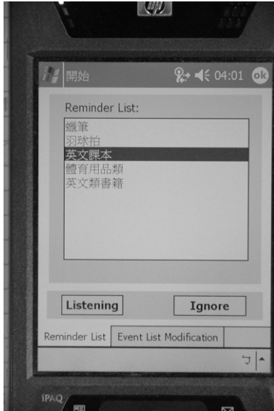
Figure 5. The reminder list sent by the server is displayed on the PDA client. The first three items are objects (crayons, badminton racquet, and English textbook); the last two are classes (sports goods and English books).
