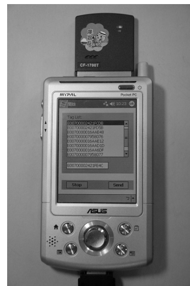
Figure 4. The CF-card RFID reader mounted on a PDA.
