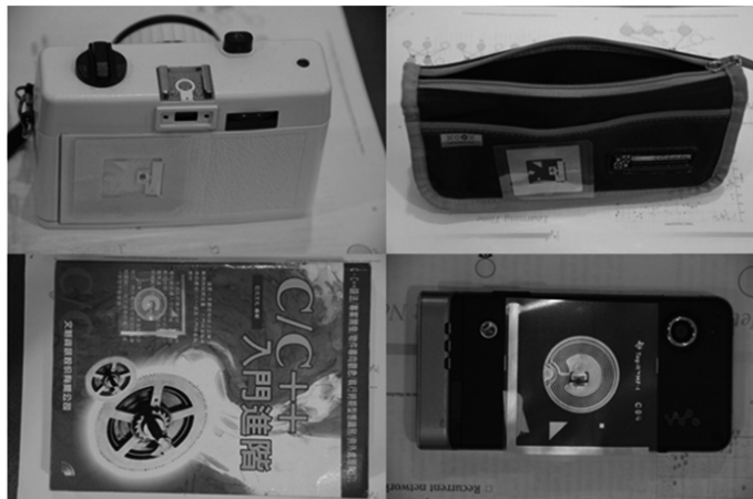
Fig. 3. Objects attached with an RFID tag.
